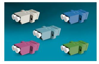
Image 2: LCD adapters in SC simplex size as offered from Datwyler – on the left side in beige for OM1 and OM2, turquoise for OM3, heather violet for OM4; on the right side for single-mode OS2 in blue (PC) and green (APC).
