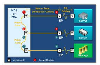
ber of connectors are involved in cross-connect (see picture above), the limits of the tight attenuation budgets can be reached sooner than expected. This fact should be weighted accordingly in a system evaluation.
