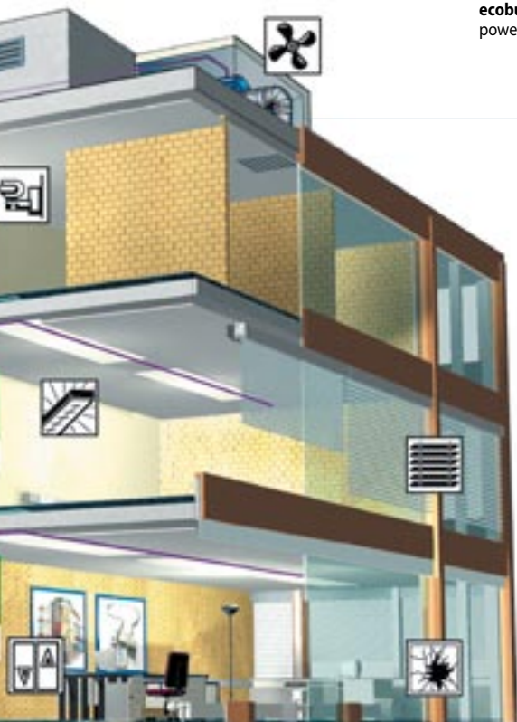
System ECO-D compact, plug-in KNX actuators with ecobus® connection technology for fast, error-free assembly in intermediate floors or suspended ceilings
