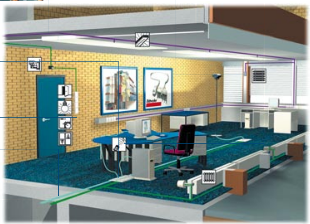
ecobus® Patch pre-assembled patch cables to connect consumers and to supply office actuators
